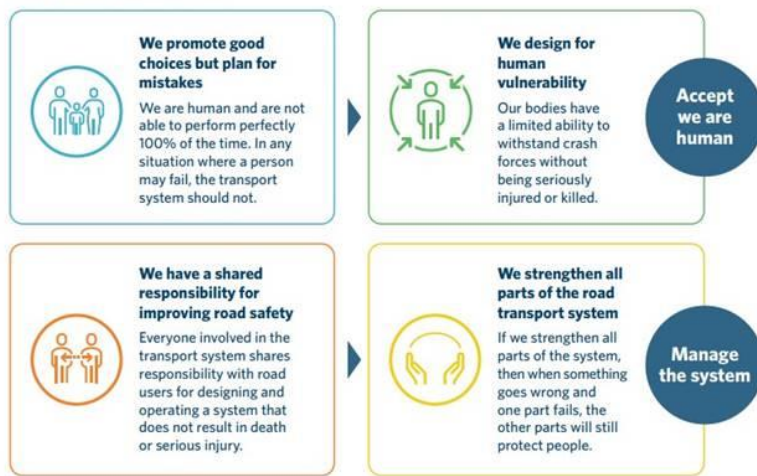
Figure 2: Safe System principles
